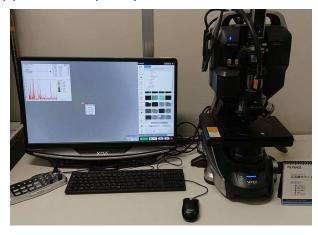
In addition to the deposition system and automatic detection device, the LIBS analysis device is also introduced to strengthen the foreign body analysis and evaluation of the coating.
